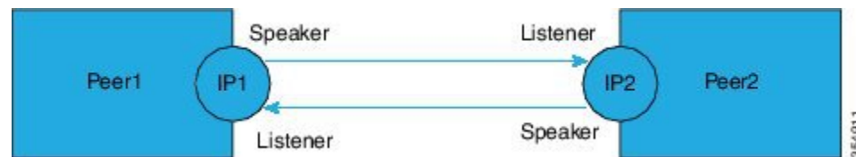
Figure 10: Bidirectional SXP Connection
