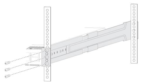
d) Tighten the 10-32 screws to 20 in-lb (2.26 N·m) or tighten the 12-24 screws to 30 in-lb (3.39 N·m) of torque.
