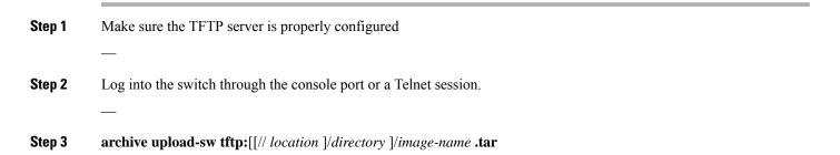
Upload the currently running switch image to the TFTP server.
