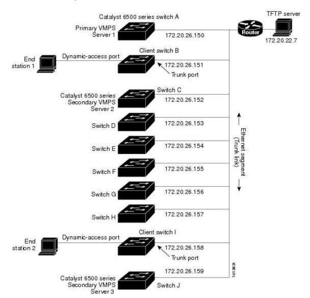
• The database configuration file is stored on the TFTP server with the IP address 172.20.22.7.
