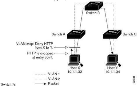
If you do not want HTTP traffic switched from Host X to Host Y, you can configure a VLAN map on Switch A to drop all HTTP traffic from Host X (IP address 10.1.1.32) to Host Y (IP address 10.1.1.34) at Switch A and not bridge it to Switch B.
