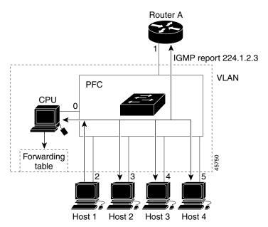
Router A sends a general query to the switch, which forwards the query to ports 2 through 5, which are all members of the same VLAN. Host 1 wants to join multicast group 224.1.2.3 and multicasts an IGMP membership report (IGMP join message) to the group. The switch CPU uses the information in the IGMP report to set up a forwarding-table entry, as shown in Table 23-1, that includes the port numbers connected to Host 1 and the router.
