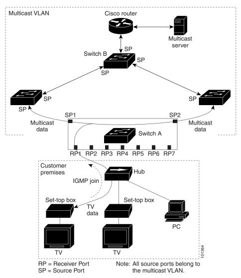
Figure 23-3 Multicast VLAN Registration Example
