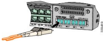
Figure 10: Network Module with SFP Modules Installed
