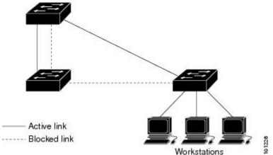
You can also create redundant links between devices by using EtherChannel groups.
