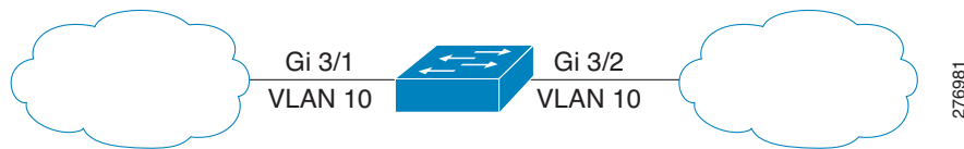
Figure 1-3 Disabling MAC Address Learning: Network Load Balancers
