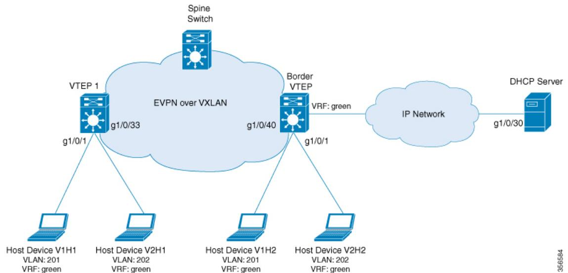
The illustration shows an EVPN VXLAN network with two VTEPs, VTEP 1 and Border VTEP. Border VTEP is connected to the DHCP server.
