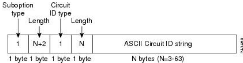
Figure 1: Suboption Packet Formats, Circuit ID Specified
