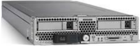
Figure 5 Cisco UCS B200 M4 Blade Server
