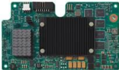
Figure 6 Cisco UCS Virtual Interface Card (VIC) 1340
