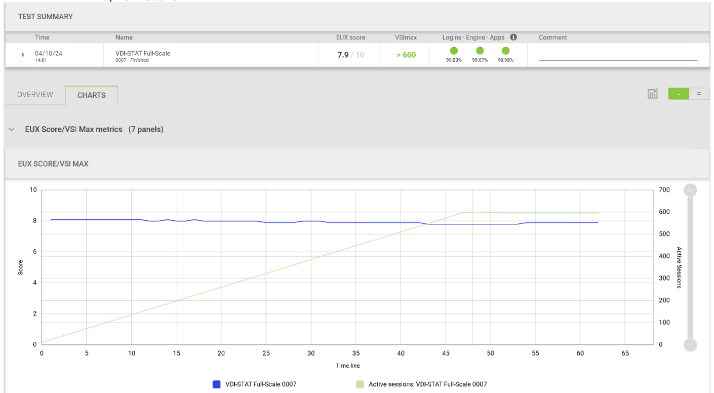
Figure 31. Full Scale | 600 Users | Citrix Virtual Apps and Desktops 2203 LTSR MCS Single-session OS machine VDAs| EUX Score
