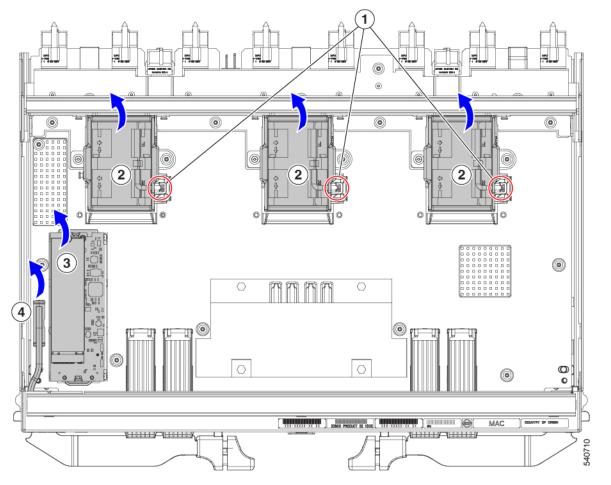
**Step 2** Remove the stiffener bracket.
