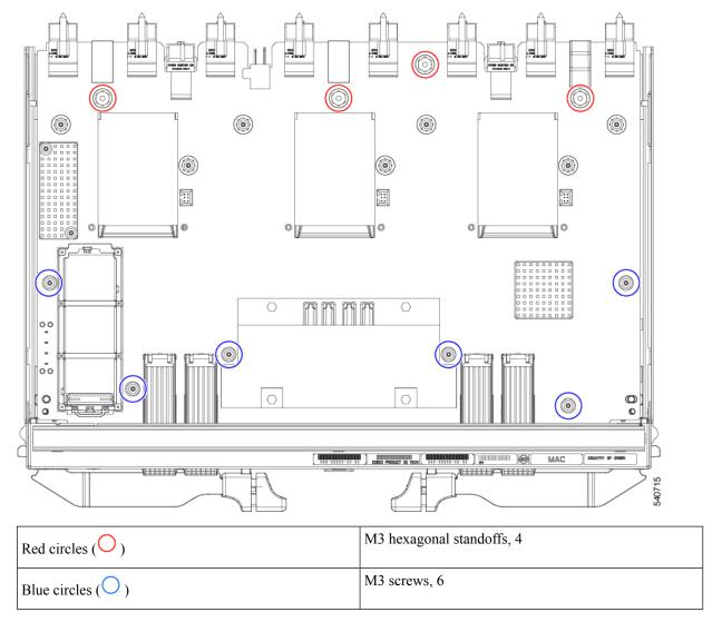
d) Grasp the PCBA and disconnect it from the sheet metal.
