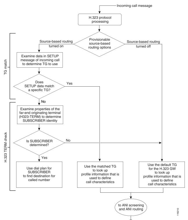
Figure 3-4 Overview of H.323 Inbound Routing Process
