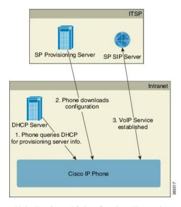
With the Cisco factory default configuration, a Cisco IP Phone automatically tries to resync to a profile on a TFTP server. A managed DHCP server on a LAN delivers the information about the profile and TFTP server that is configured for preprovisioning to the device. The service provider connects each new Cisco IP Phone
