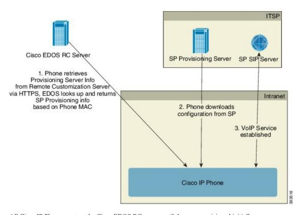
All Cisco IP Phones contact the Cisco EDOS RC server until they are provisioned initially.
