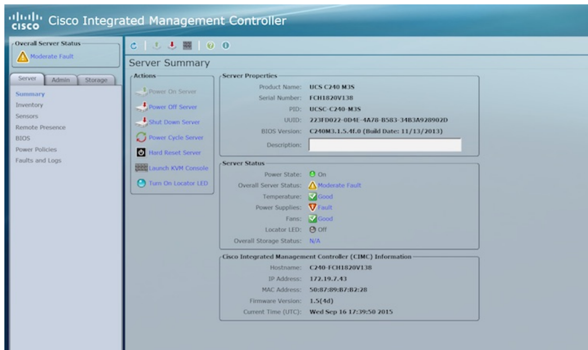
Figure 9: Cisco Integrated Management Controller Interface
