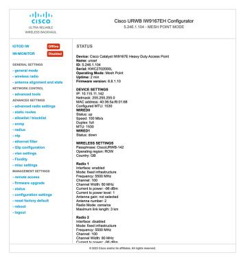
7. To establish a wireless connection between devices, set the same operating frequency in radio devices.
