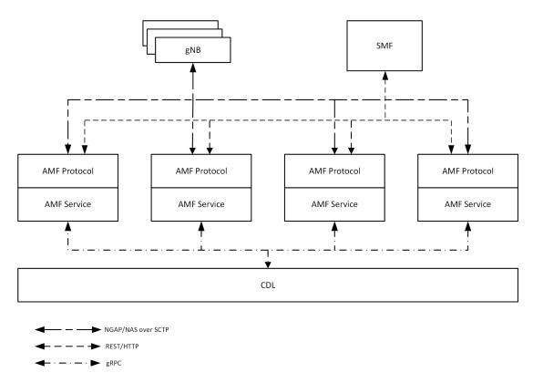
The CDL is deployed as an independent entity which acts as a session store for all the instances of AMF during AMF scaling. Each AMF instance performs the following:
