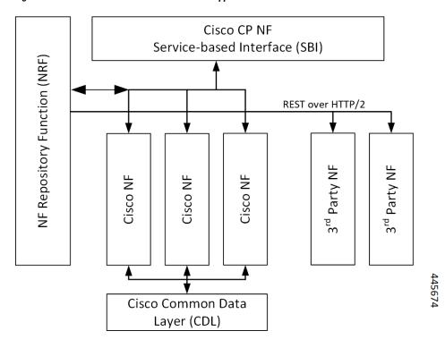
Figure 4: Cisco CP NF Service-based Architecture Support
