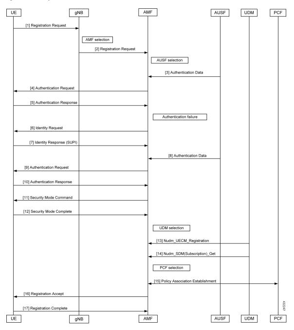
Figure 30: UE Identity Procedure for Authentication Failure Call Flow
