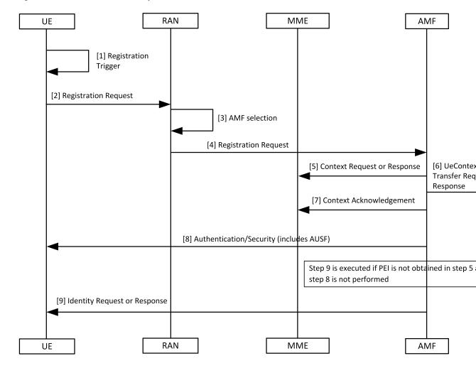
Figure 64: Idle or Connected Mode Mobility Call Flow
