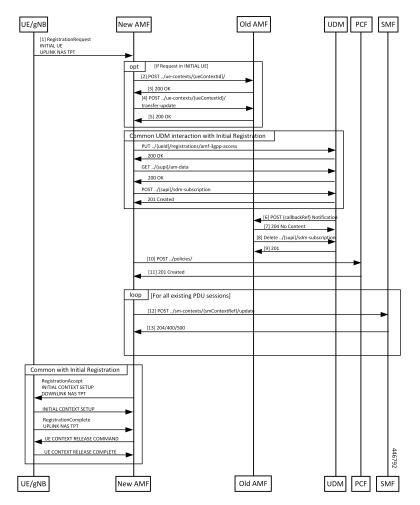
Figure 40: Registration with AMF Change Call Flow
