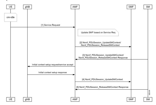
Figure 67: Idle Mode Call Flow
