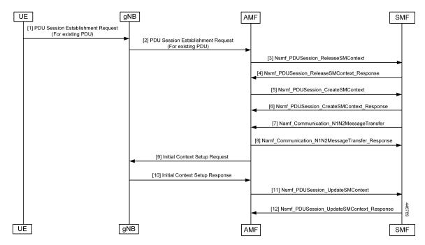
The UE receives data services through a PDU session, which is a logical connection between the UE and the core network. The PDU Session Establishment procedure describes the procedures by which UE establishes a PDU session for accessing data services. In 5G, the UE can establish a PDU session when service is needed.
