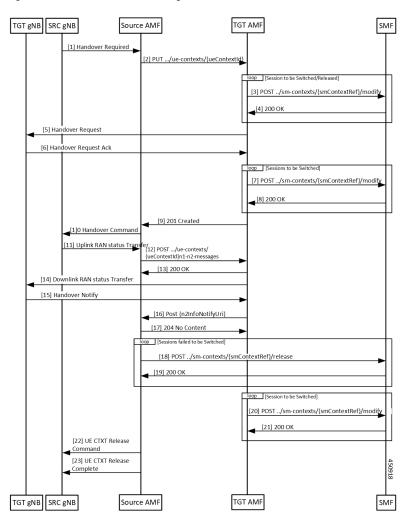
Figure 47: N2 Handover with AMF Change Call Flow
