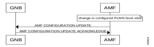
Changes in the slice configuration per PLMN is notified to GNBs using AMF configuration update message.
