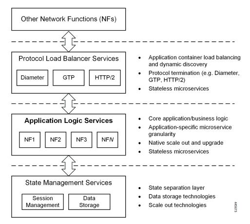
Figure 3: Control Plan Network Function Tiered Architecture
