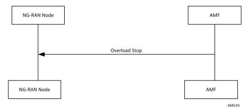
After the overload situation is resolved, the AMF sends an Overload Stop Message to the NG-RAN node indicating that the AMF is ready to resume the process the sessions.
