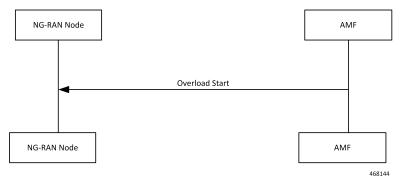
When the overload control is configured and the congestion threshold is reached, the AMF sends an Overload Start Message to the NG-RAN Node.
