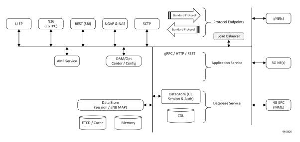
The SCTP endpoint (EP) pod type supports the SCTP interface between the AMF and gNB. Only a single SCTP EP pod is run at a time. In addition to a GUAMI, the SCTP bind address is also unique to an AMF. If multiple SCTP EPs are run, they have to bind to different SCTP addresses, at which time they would not be part of the same AMF.
