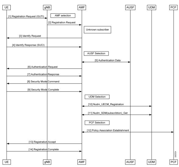
Figure 44: UE Identity Procedure for Unknown GUTI Registration Call Flow
