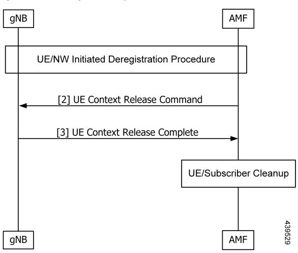
Figure 36: UE or NW-Initiated Deregistration followed by UE Release Procedure Call Flow
