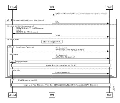
Figure 45: N1N2 Message Transfer Request Call Flow
