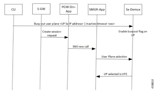
In continuation to the previous call flow, this call flow describes about the clearing of the idle subscriber based on the busy-out inactivity- timeout:
