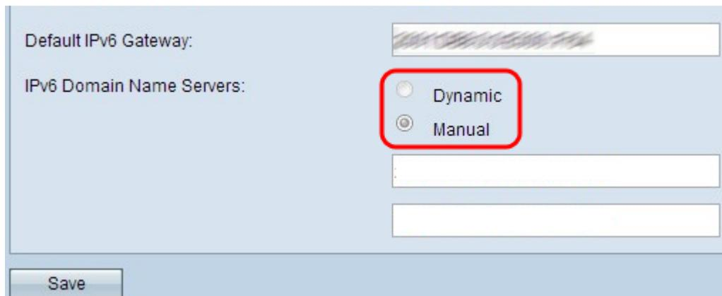
This screenshot is similar to the previous one but highlights the 'Dynamic' and 'Manual' radio buttons with a red rectangular box. The 'Manual' option is selected. A 'Save' button is visible at the bottom left of the configuration area.
