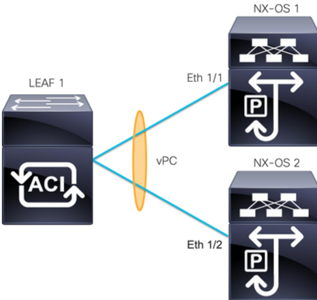
ACI LEAF 1: interfaccia Ethernet 1/1 ed Ethernet 1/2, Port-Channel 5 e vPC 343
