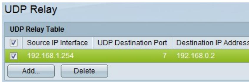
The screenshot shows a window titled "UDP Relay" with a table labeled "UDP Relay Table". The table has three columns: "Source IP Interface", "UDP Destination Port", and "Destination IP Address". There is one row of data with a checkmark in the first column, the value "192.168.1.254" in the second column, the value "7" in the third column, and the value "192.168.0.2" in the fourth column. Below the table are two buttons: "Add..." and "Delete".
