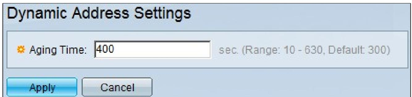
The image shows a screenshot of the 'Dynamic Address Settings' configuration window. The window has a light blue header with the title 'Dynamic Address Settings'. Below the header, there is a text input field for 'Aging Time' with the value '400' entered. To the right of the input field, it says 'sec. (Range: 10 - 630, Default: 300)'. At the bottom of the window, there are two buttons: 'Apply' and 'Cancel'.
