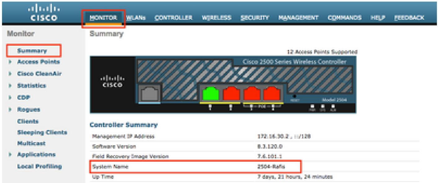
The screenshot shows the Cisco WLC Monitor interface. The 'MONITOR' tab is selected in the top navigation bar. In the left sidebar, the 'Summary' option is highlighted. The main content area displays a 'Summary' section for a 'Cisco 2500 Series Wireless Controller'. Below this is a 'Controller Summary' table with the following data:
