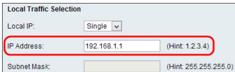
The screenshot shows the 'Local Traffic Selection' form. The 'Local IP:' dropdown menu is set to 'Single'. The 'IP Address:' field contains the value '192.168.1.1' and is highlighted with a red box. The 'Subnet Mask:' field is empty. There are hints for the IP address (1.2.3.4) and Subnet Mask (255.255.255.0).
