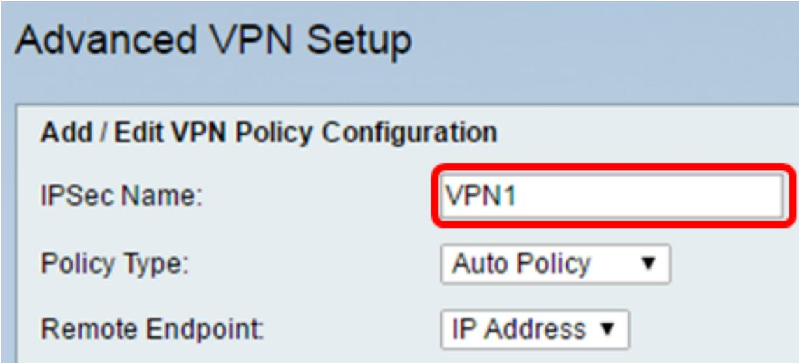
The screenshot shows the 'Advanced VPN Setup' interface, specifically the 'Add / Edit VPN Policy Configuration' section. It contains three fields: 'IPSec Name' with a text input field containing 'VPN1', 'Policy Type' with a dropdown menu set to 'Auto Policy', and 'Remote Endpoint' with a dropdown menu set to 'IP Address'. The 'IPSec Name' input field is highlighted with a red box.
