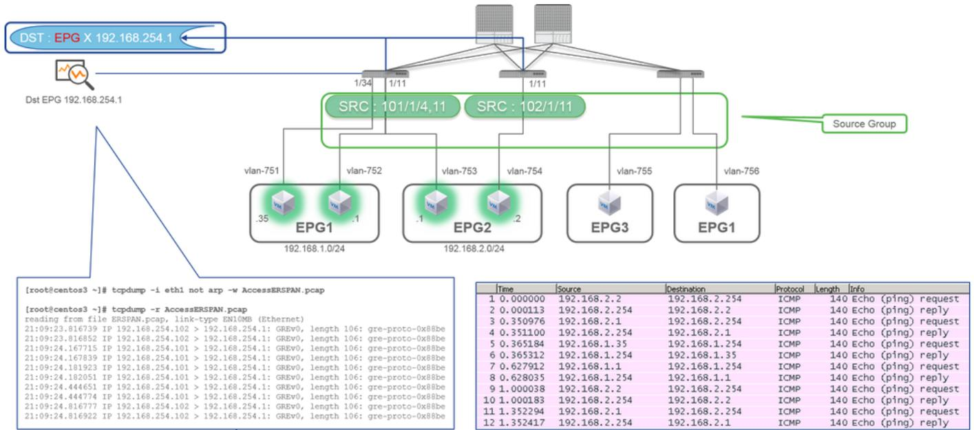
※ ERSPAN = GRE encap'ed packet = Src/Dst are GRE IP
