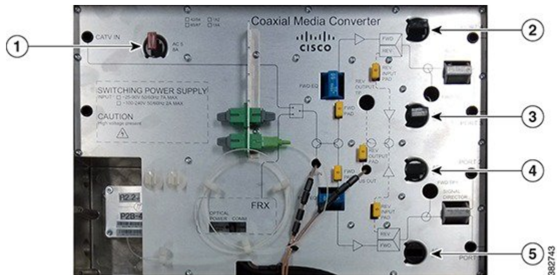
Figure 37: Location of AC Shunts on the Cisco CMC
