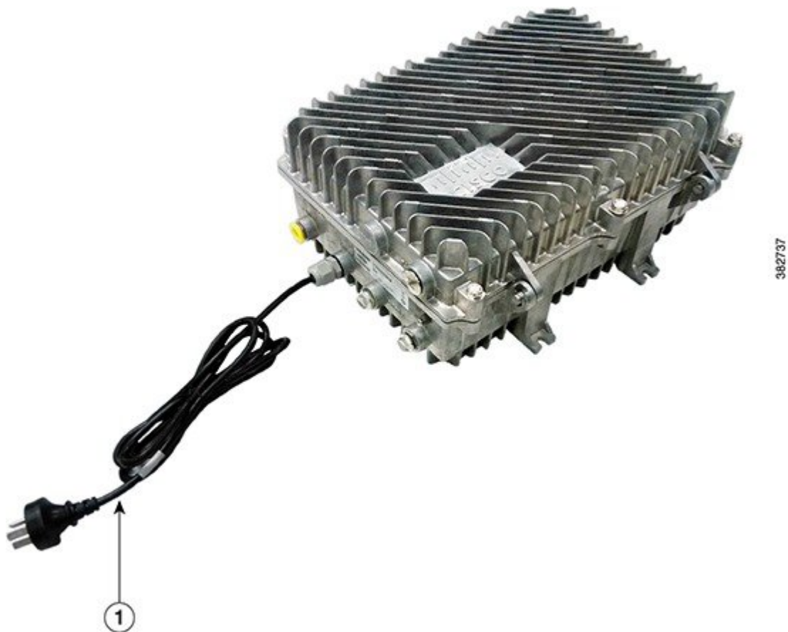
Figure 35: Connecting 220VAC Power to the Cisco CMC
