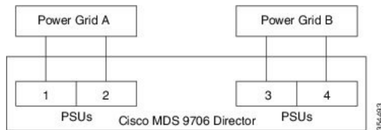
Figure 26: Cisco MDS 9706 Grid-PSU Connections
