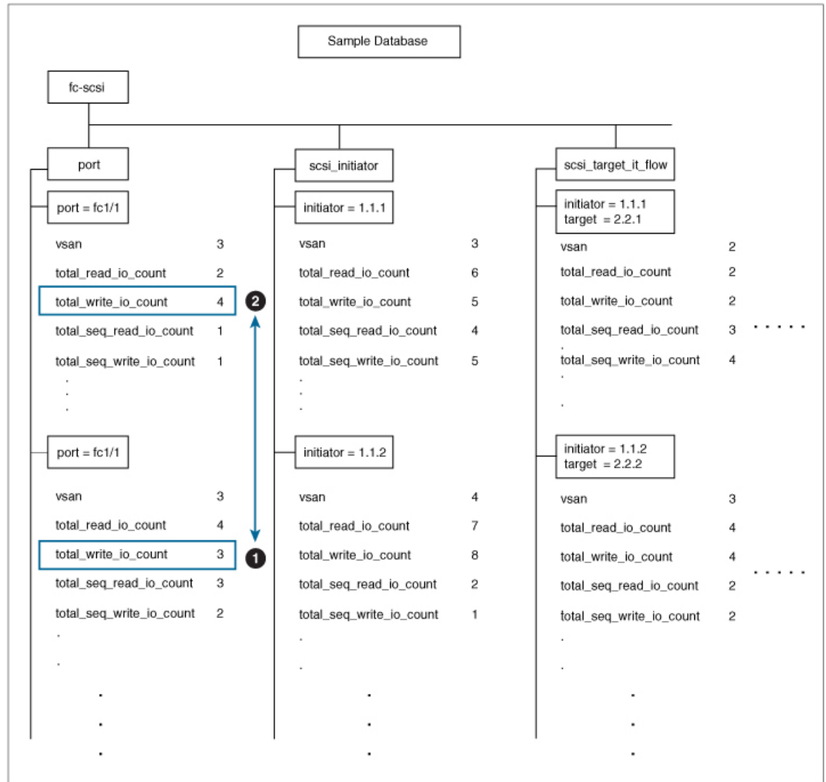
Figure 30: Flow Metrics of an Initiator's Total Write IO Count That Belongs to Port FC1/1 and VSAN 3 With the Output Sorted
