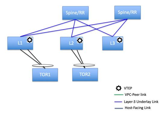
• ToR switches directly connected to the leaf switches. vPC pairs are not configured for the leaf or ToR switches.
