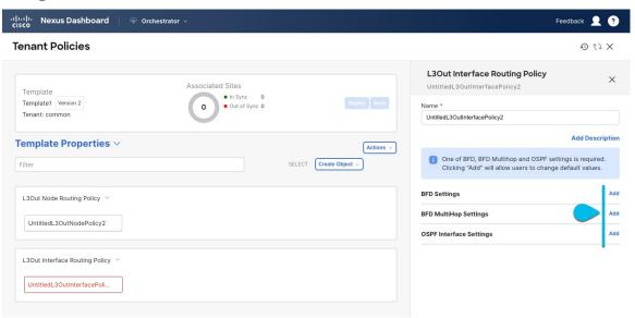
BFD settings – provides forwarding failure detection between ACI fabric border leaf switches that are configured to support peering router connections.
