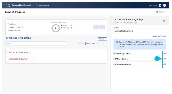
• **BFD Multi-Hop Settings** – provides forwarding failure detection for destinations with more than one hop. In this case, a multi-hop session is created between the source and destination instead of the interface like in single-hop scenarios.
