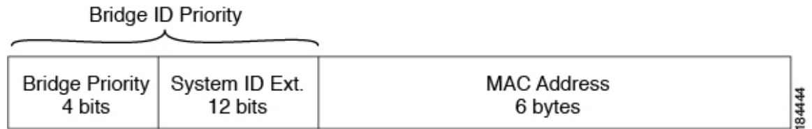
Figure 6: Bridge ID with Extended System ID
