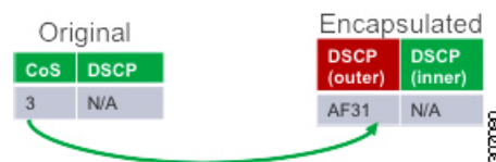
Figure 37: Copy of Priority from Layer-2 Frame to VXLAN Outer Header
