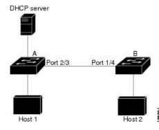
If you configure interfaces as trusted when they should be untrusted, you may open a security hole in a network. If device A is not running DAI, host 1 can easily poison the ARP cache of device B (and host 2, if you configured the link between the devices as trusted). This condition can occur even though device B is running DAI.
