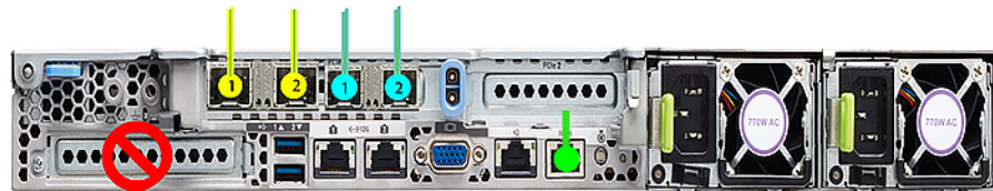
Intel X710 quad-port 10G / Cisco-Intel E810XXVDA4L 4x25/10G
