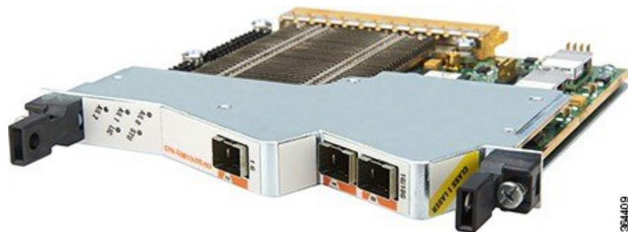
Figure 4: Cisco 6 Gbps Wideband Shared Port Adapter Faceplate
