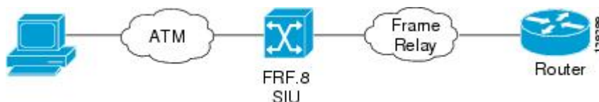
Figure 2 Frame Relay-to-ATM Interworking
