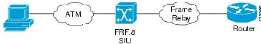
Figure 2 Frame Relay-to-ATM Interworking
