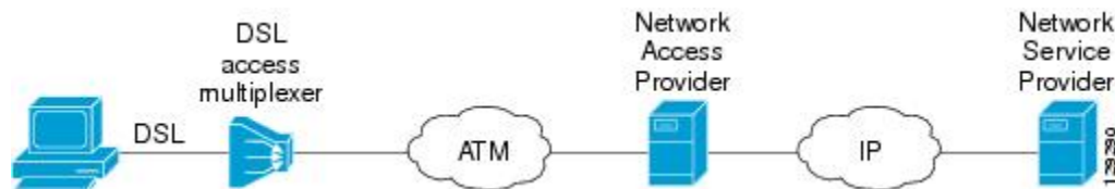
Figure 3: PPP over ATM SVC Terminating at a Network Access Provider
