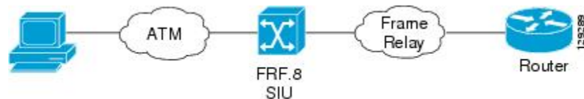
Figure 2: Frame Relay-to-ATM Interworking
