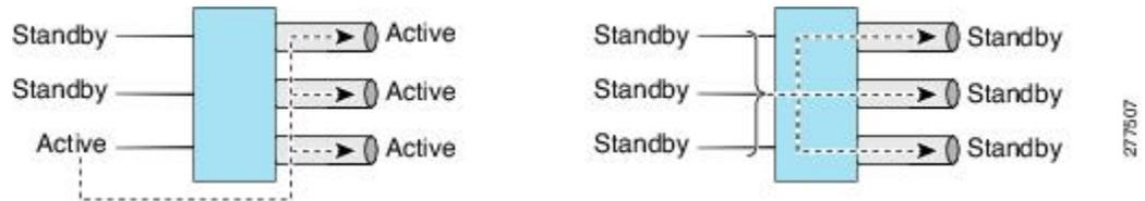
VPLS decoupled mode is when all pseudowires in the VFI are always active and the attachment circuit state is independent of the pseudowire state. This mode provides faster switchover time when a platform does not support pseudowire status functionality, but extra flooding and multicast traffic will be dropped on the PE with standby attachment circuits. See the figure below.
