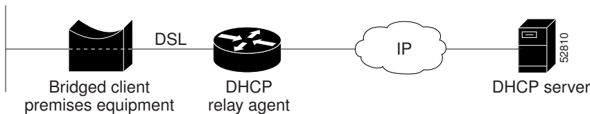
Figure 18 Network Topology Using ATM RBE and DHCP
