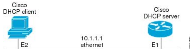
Figure 10 Topology Showing a DHCP Client with a Gigabit Ethernet Interface
