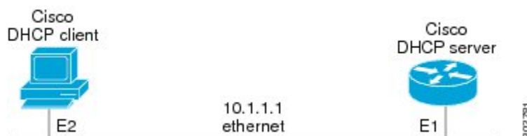
Figure 7: Topology Showing a DHCP Client with a Gigabit Ethernet Interface
