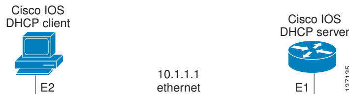
Figure 11 Topology Showing DHCP Client with GigabitEthernet Interface
