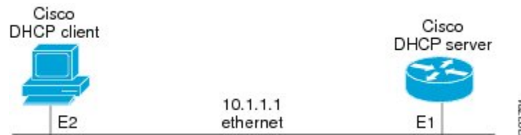
Figure 4: Topology Showing a DHCP Client with a Gigabit Ethernet Interface
