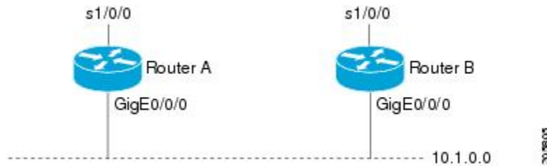
Figure 1: Topology for IP-Routing Support
