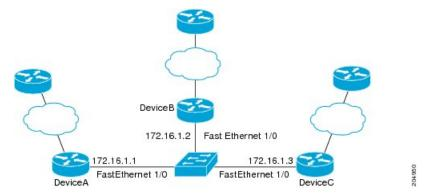
When Fast Ethernet interface 1/0 on RouterB fails, BFD will no longer detect Router B as a BFD neighbor for RouterA or for RouterC. In this example, Fast Ethernet interface 1/0 has been administratively shut down on RouterB.
