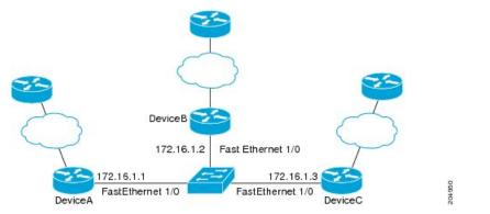
The example, starting in global configuration mode, shows the configuration of BFD.
